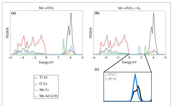
$\textbf{Figure 2.} \ Computed \ PEDOS \ for \ (a) \ stoichiometric \ Mo-doped \ TiO_2 \ anatase \ and \ (b) \ reduced \ Mo-doped \ TiO_2 \ anatase, with one oxygen \ vacancy. \ Panel \ (c) \ shows \ the \ occupied \ Ti^{3+} \ and \ Mo^{5+} \ states \ which \ emerge \ in \ the \ band \ gap \ after \ vacancy \ formation.$
